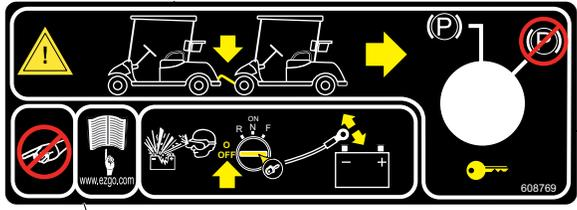
KEEP HANDS OUT    READ THE MANUAL REPLACEMENT AVAILABLE AT [www.ezgo.com](http://www.ezgo.com)    TO REDUCE POSSIBILITY OF BATTERY EXPLOSION TURN KEY TO 'OFF' BEFORE DISCONNECTING OR CONNECTING BATTERY WIRES
