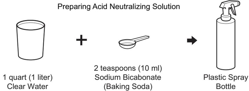
The correct cleaning method is to spray the top and sides of the batteries with a solution of baking soda and water. Apply this solution with a plastic spray bottle. The solution is 2 teaspoons (10 ml) sodium bicarbonate (baking soda) mixed with 1 quart (1 liter) of water. Spray the solution on all metal components near the batteries also.
