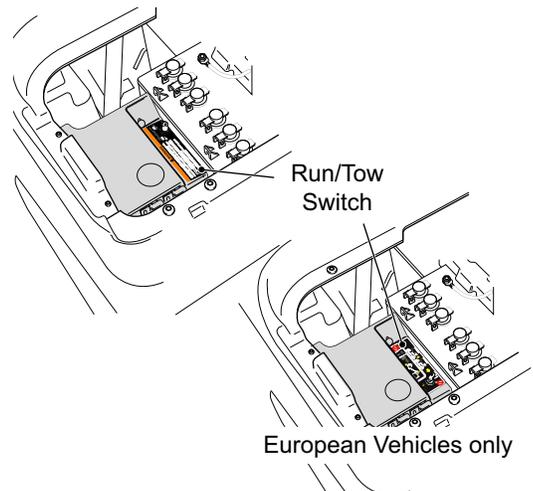
Figure 3 Run/Tow Switch
