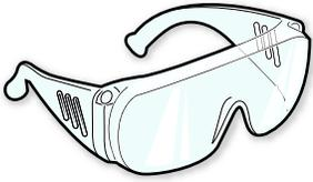
*Always wear a safety shield or approved safety goggles when you add water or charge the batteries.*
