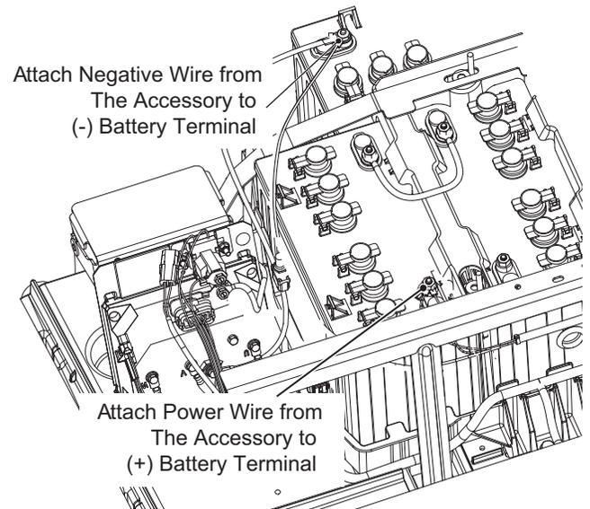
Figure 2 Accessory Wires to Battery Pack Attachment
