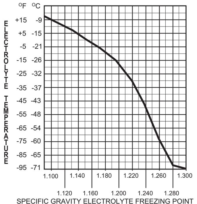
Figure 9 Freezing point of electrolyte
